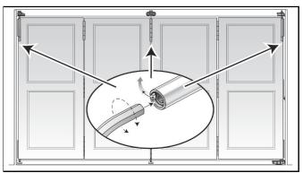
• Install the factory-provided screws into the bottom of the upper pin heads.
