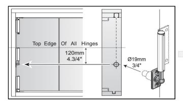
• Set the first slab into place, and attach the wall pivot hinges to the door slab. Spacer blocks may be needed to elevate the slab to the correct position.
