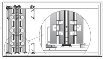
Make final adjustments to the carrier pin nut to ensure smooth operation.
