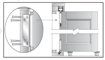
Make the proper adjustments to the upper and lower pivots until the door slab is level.
