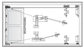
• Continue by setting the additional slab(s) into place and install using the pivot hinges, upper track carrier and lower track pivots.
